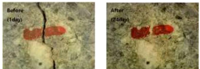
(b) specimen that containing coated silica sand with self-healing ingredient
