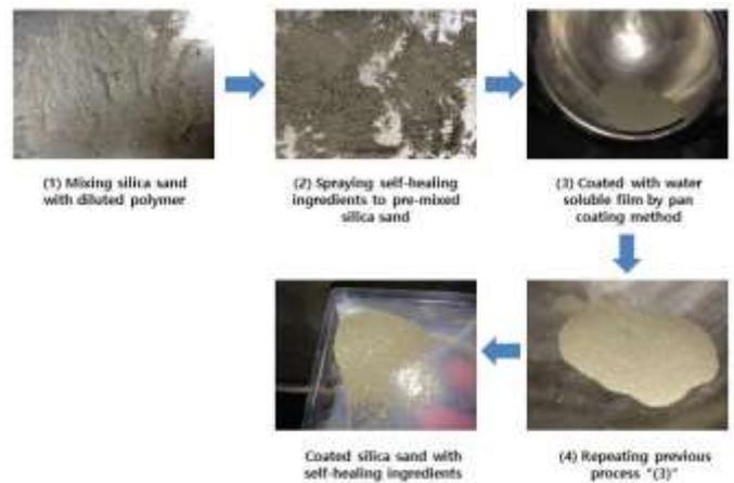
Fig.2. The method of coating and using materials.
