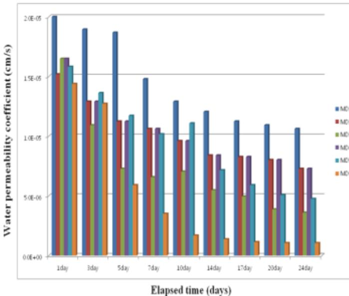
Fig. 5. shown the result. This result indicated that the range of water permeability of all specimens is 1.4-2.0 x 10 (cm/s) after the introduction of crack.
