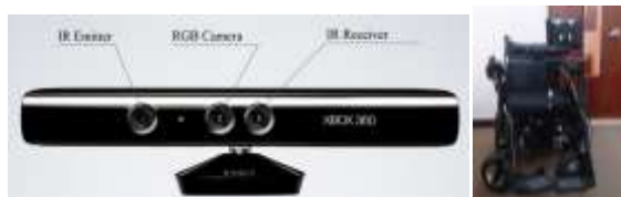
Figure 1. Microsoft Kinect device (left) and electronic wheelchair with Kinect camera (right).
