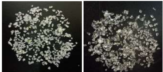
Figure 3. Glass beads before (a) and after (b) dip-coated with Ag-TiO 2 -SiO 2
