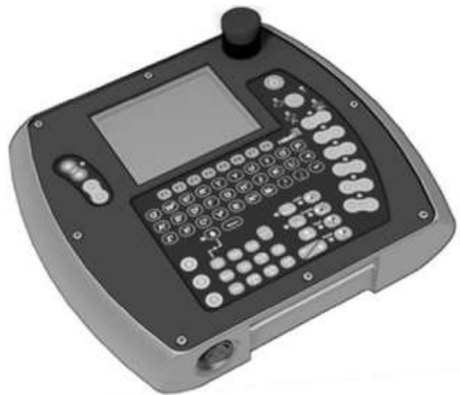
Figure 6. Remanufactured handheld terminal for industrial robots
