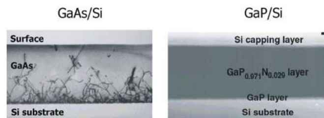
Figure 4. Transmission Electron Microscopy (TEM) images of lattice mismatch due to dislocations formed in the GaAs layer grown on Si (Left), Contrarily GaP/GaN layers can be formed on Si without any threading dislocations [9]
