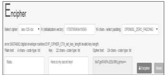
Figure 3. Catch an error message complete fields and result for symmetric cryptography encryption operation.
