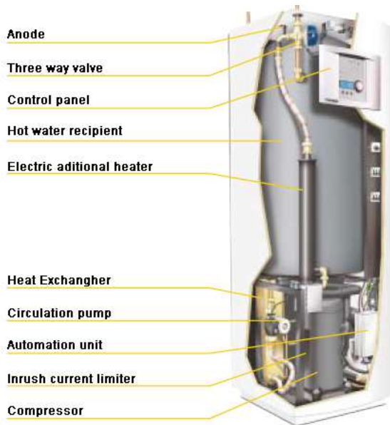
Fig.5 Heat Pump scheme (source: processed picture)
