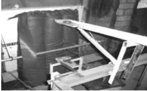
Figure 8. Tested composite wall.
