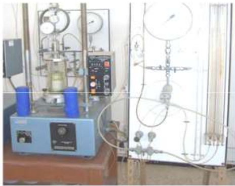
Figure 2a. Triaxial testing.
