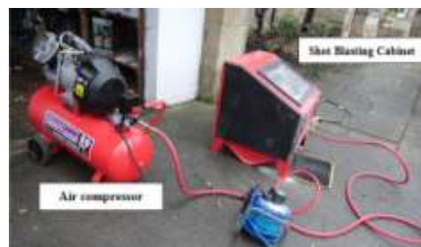
Figure 2. The abrasive cleaning system.
