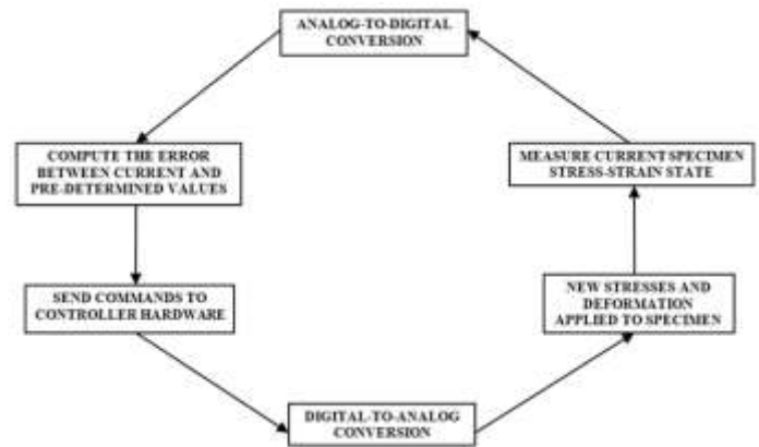
Figure 2. Closed Feedback Control Loop Processed during the Execution of The Controller Software
