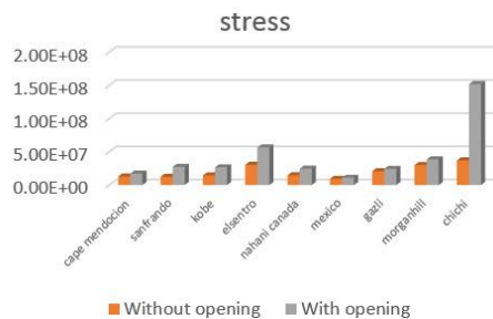
Figure 9. Stresses in chimneys with and without opening.
