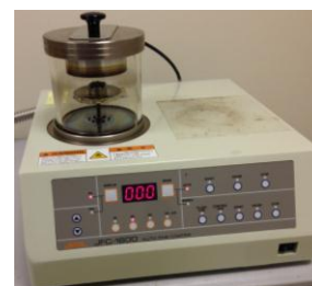
Figure 4: Apply Conductive Coating
