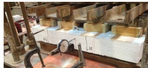
Figure (5): Horizontal dial gauges for slippage measurements.
