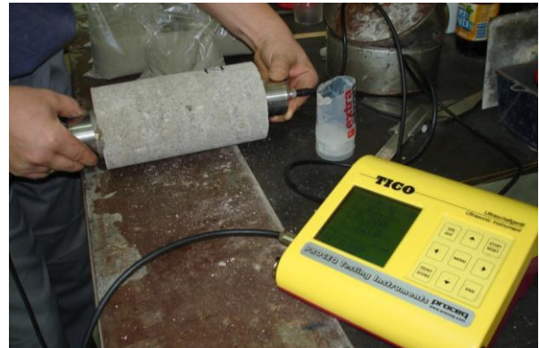
Figure 2. Measurement of ultrasound pulse velocity
