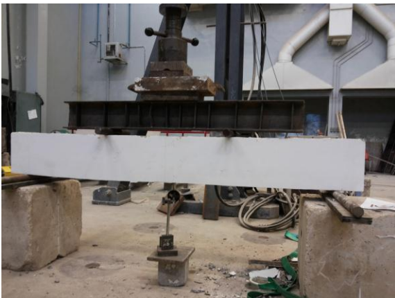
Fig. 4: Experimental set up and crack monitoring
