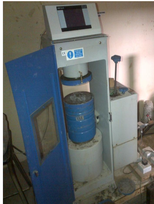
Plate 2.2 ADR Touch Compressive Testing
