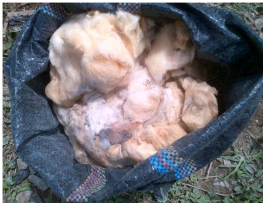
Plate 2.1: Glass Wool Fibre
