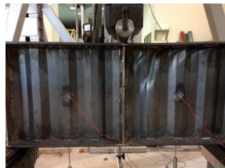
Fig. 5: Profile of beam A12-410-30 after loading-buckled panel.
