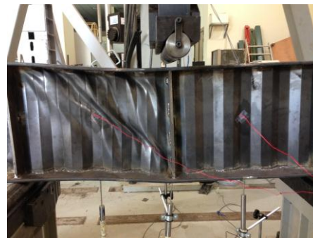
Fig. 5: Profile of beam A12-410-30 after loading-buckled panel.
