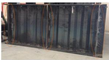
Fig. 3. Profile of test beam with stiffeners.
