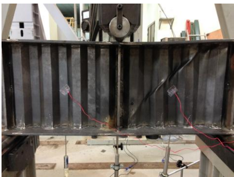
Fig. 11: Profile of beam A12-410-45 a) after loading. b) buckled panel.
