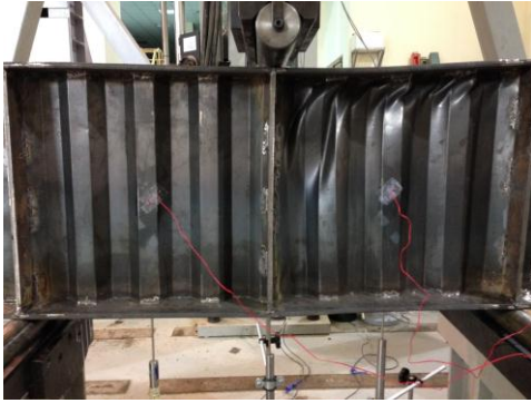
Fig. 7: Profile of beam A12-505-45 after loading-buckled panel.
