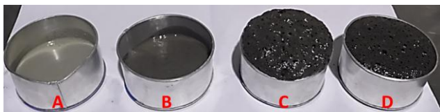
Figure 5. Slurries with KOH after 5:55 min.
