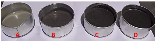
Figure 3. Slurries with KOH after 4:39 min.
