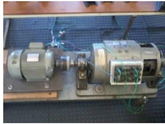
Figure 3. Generator-group: DC motor and an induction generator.
