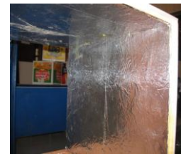
Fig. 2. Wooden box fabricated with heat proof material
