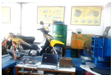
Figure 14: Honda Wave RS is mounted on a dynamometer.
