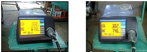
Figure 18: Parameters measured emission results when using TI - CDI ignition and overseas original CDI ignition.
