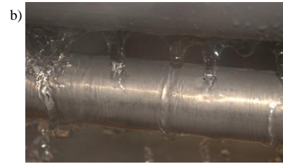
Figure 21. Feeder film with 20 LPM on a) rough surface tube, b) smooth surface tube.
