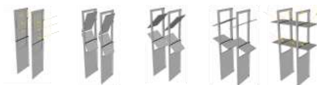
Figure 7. Transformation Procedure of the Proposed Façade System
