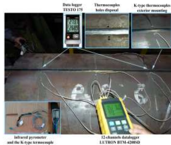
Figure 4. Temperature measurement system outside the pipeline
