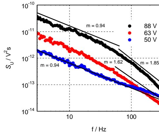
Figure 7. Low frequency noise spectral density of sample after applying the process of thermal stressing.
