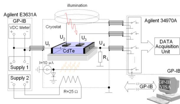
Figure 1. Experimental setup for the transport and the noise characteristics measurements.
