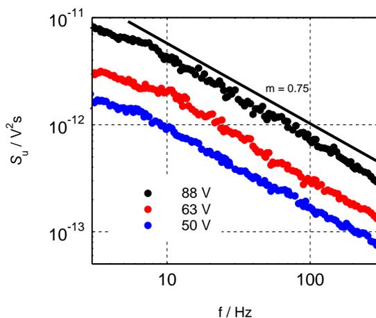
Figure 6. Low frequency noise spectral density of sample before applying the process of thermal stressing.
