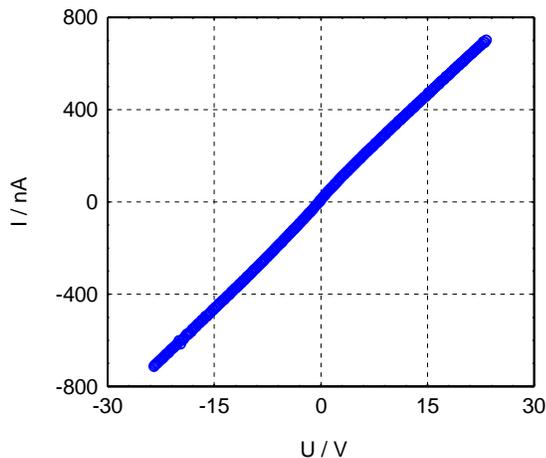
Figure 3. IV characteristic of the sample after applying the process of thermal stressing.
