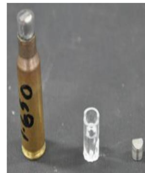
Figure 2: Completed projectile (left), sabot (middle) and FSP (right)
