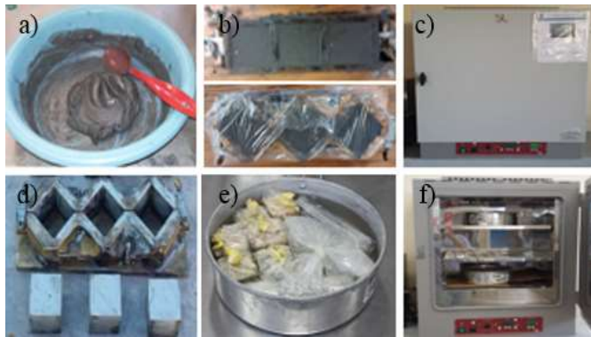
Figure 1. Preparation of mortars process: a) preparation of mixture; b) filling of molds; c) acceleration of curing process at 80 °C; d) unmolding; e) specimens in watertight containers with water; f) curing at 80 °C.
