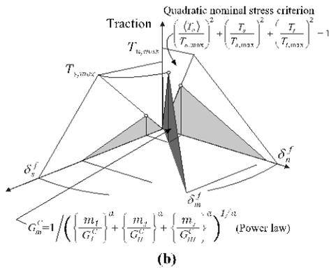
Figure 5. (a) Bilinear cohesive law, (b) CZM mixed mode in ABAQUS™.
