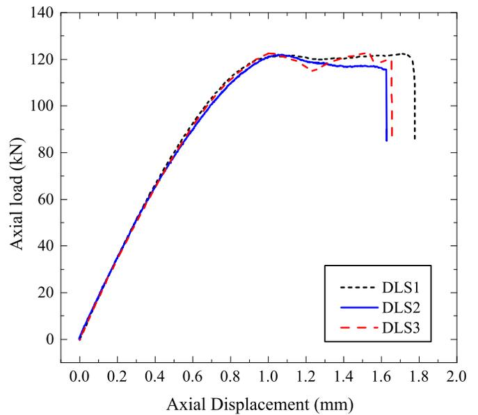
Figure 4. Double lap shear specimens test results
