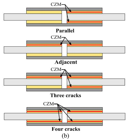
Figure 6. (a) The boundary conditions and general mesh of the DLS joints, (b) different investigated failure modes.
