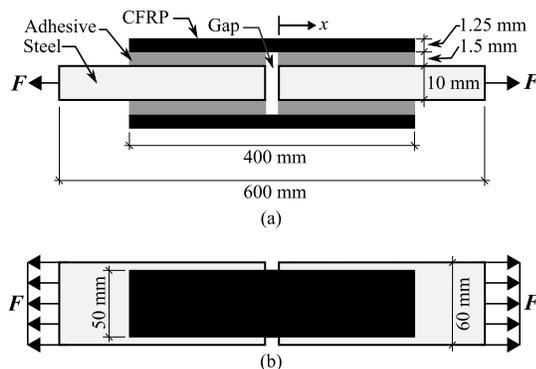
Figure 3. DLS joints: (a) side-view, (b) top-view
