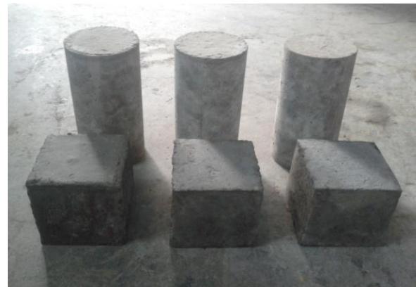
Figure 2. Casting of Geopolymer concrete cubes and cylinders
