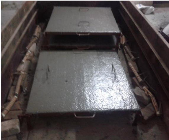
Figure 4. Heat Curing of Reinforced Geopolymer concrete Slabs.
