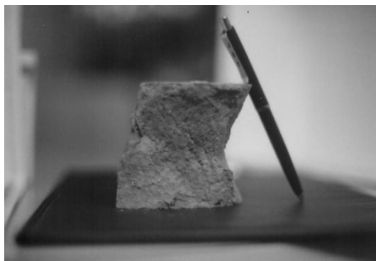
Figure 2. Compressive test and tested cubic adobe sample
