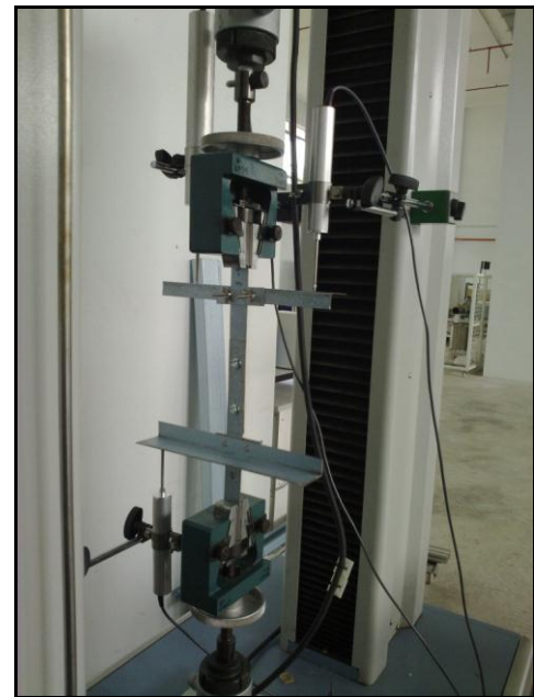
Figure 4. Single shear connection test setup
