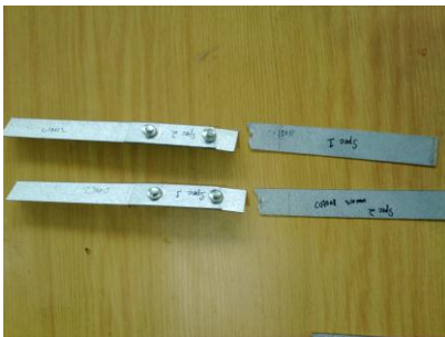
Figure 9. Net section tension failure (S208/12)
