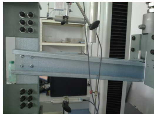
Figure 12. No buckling failure (BC4)
