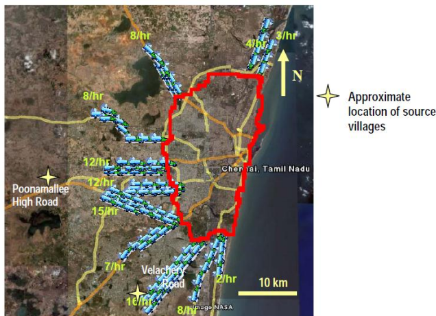
Figure 2. Movement of peri-urban groundwater towards Chennai city (Sreenivasan 2008)
