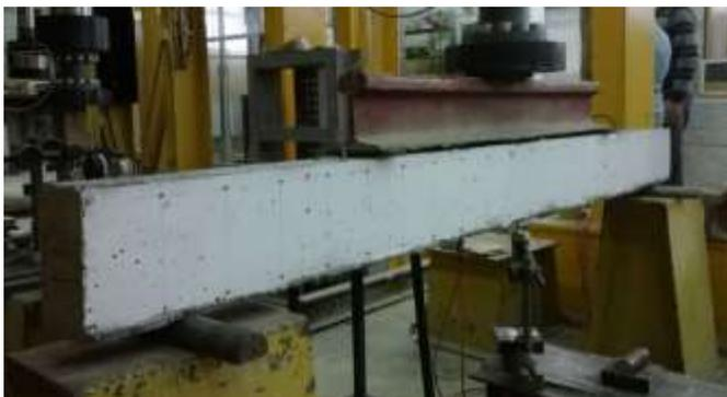
Figure 2. Prepared laboratory station. Beam located under the hydraulic press and prepared for survey.
