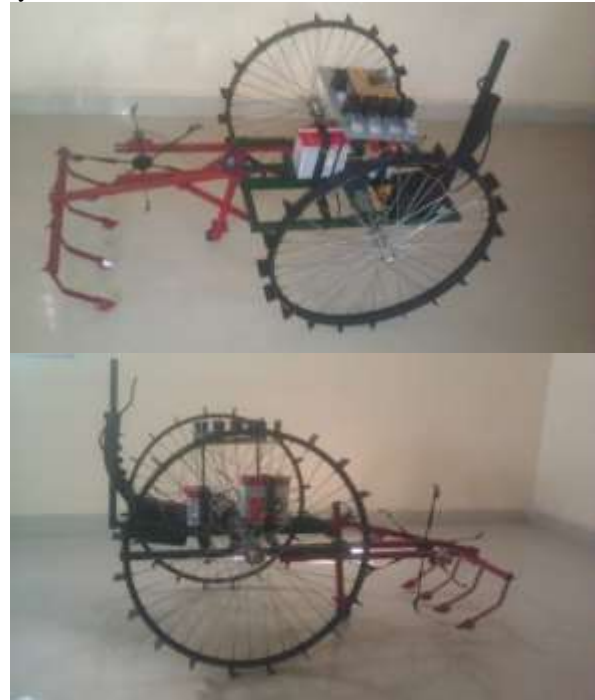
FIGURE 5. The mobile robot with a spraying system
