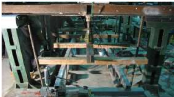
Figure 2. Loading mode and experimental layout of the truss girders
