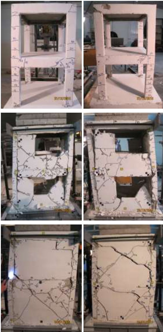
Fig 5. Specimen 1 (reference specimen), Specimen 2 (window opening) and Specimen 3 (no window opening) can be seen at the end of the test, respectively.
