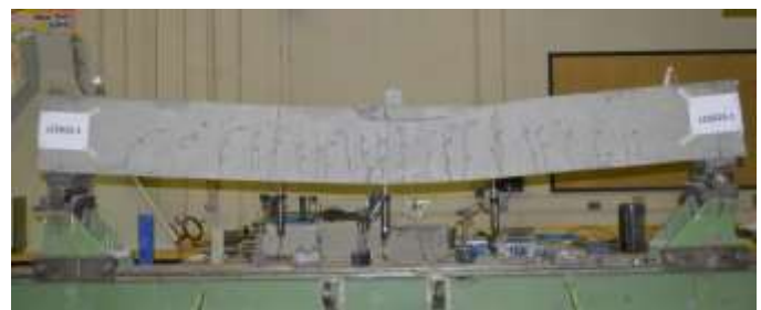
Figure 4. Mode of failure for beam L25R25-1
