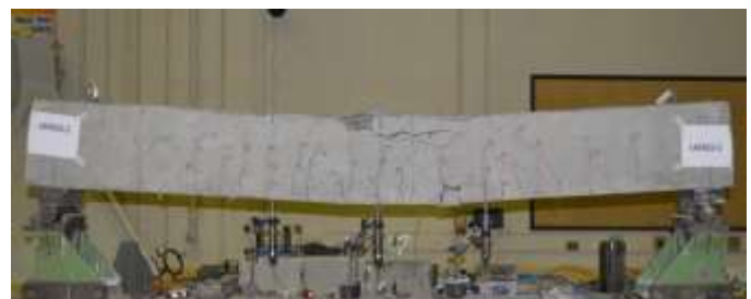
Figure 5. Mode of failure for beam L45R25-2
