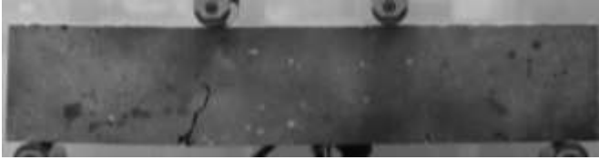
Fig. 1. A failed concrete beam sample
