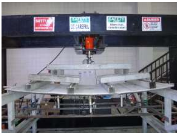
Figure 4 Testing of a PSSDB floor under bending loads
