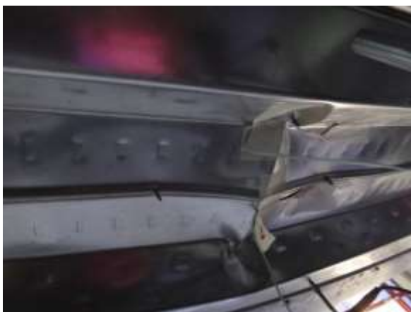
Figure 5 Local buckling for CS sample
