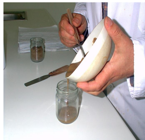
Figure 2. Saturation of soil with distilled water (TGAE, 2012)
