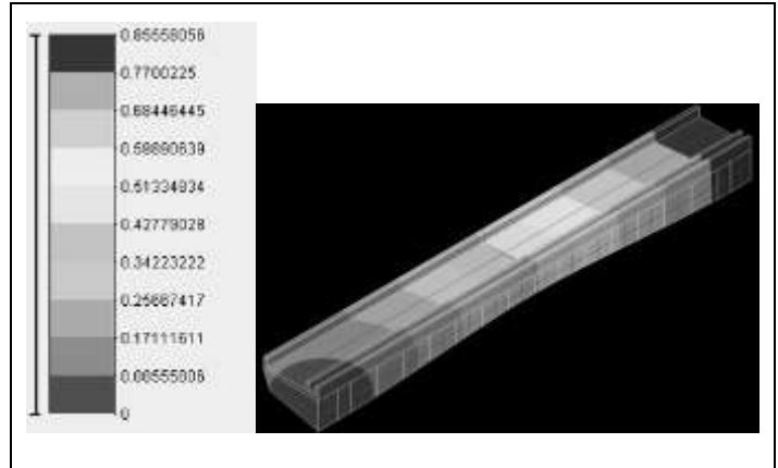
Figure 8a) Results of the finite element model: overall nodal displacements;
