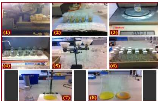
Figure 3 Powder samples collection and titration process
