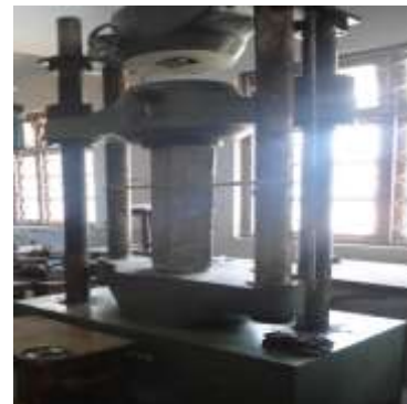
Figure 3. Complete test set up in UTM
