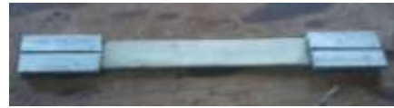
(b) Coupons prepared from GFRP sheets for testing All dimensions are in mm
