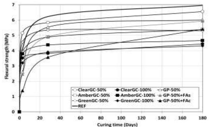
Figure 3. Flexural strength vs. curing time.
