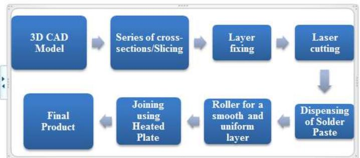
Figure 1: Composite metal foil manufacturing process
