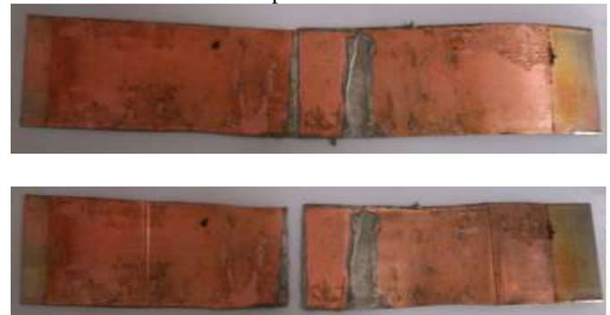
Figure 2: Failure Modes of Lap-Shear Specimens
