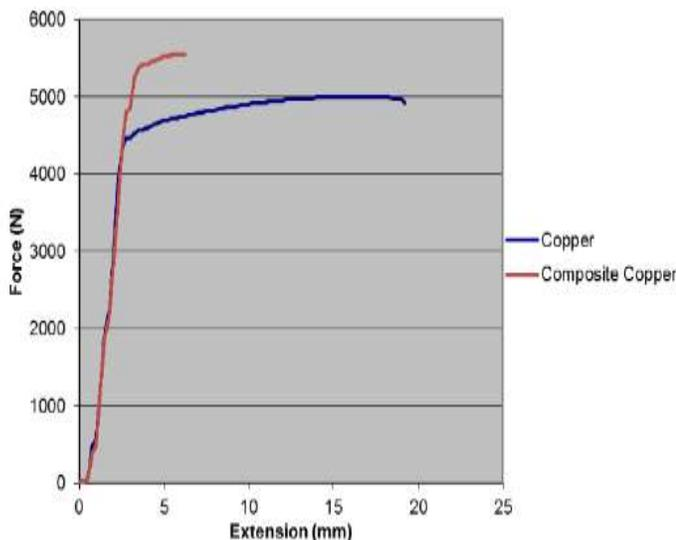
Figure 3: Comparative tensile test results
