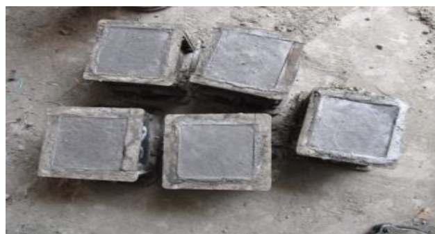
Figure 1Casting of specimens
