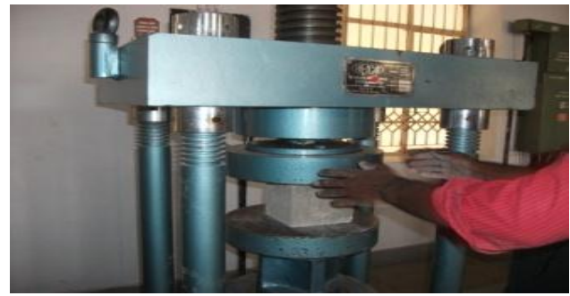
Figure 3 Compressive strength test
