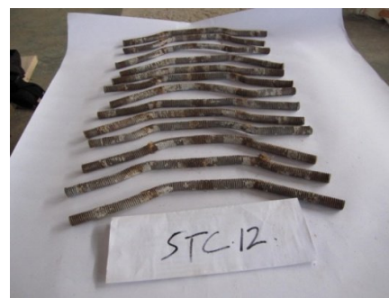
Figure 8 The hinge plastic of bolt
