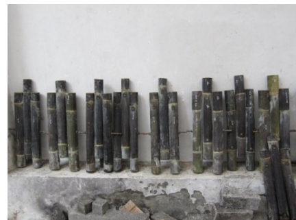
Figure 7 Specimens of three-component bamboo
