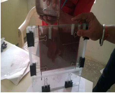
Figure 3. Pouring of Mixture in the Mould
