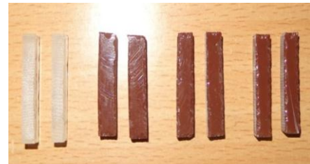
Figure 5. Specimens for 2-body wear test
