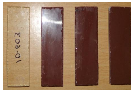
Figure 7. Specimen for 3-body wear test
