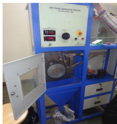
Figure 8. Dry Sand Abrasion Tester for 3-body wear testing
