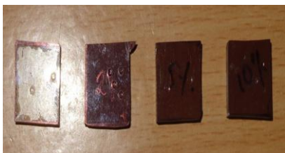
Figure 13. Specimen for hardness test.
