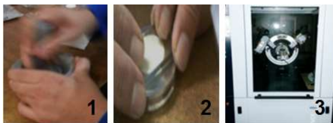
Figure 4.- Sample preparation procedure for X-ray diffractometer.
