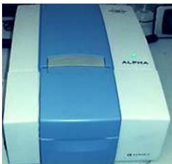
Figure 5.- infrared spectroscopy equipment, FTIR- Alpha 1, brand: Bruker.
