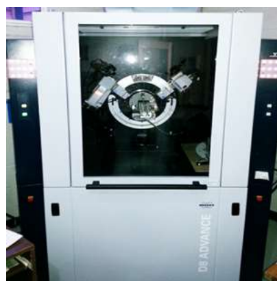
Figure 2.- X-ray diffractometer D8 Advance, brand: Bruker.
