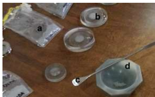
Figure 3.- Minor equipment and sample preparation in X-ray diffractometer instrument; a) geopolymer sample, b) sample holder, c) spatula d) agate mortar and spatula.
