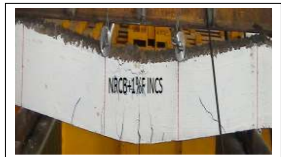
Figure 11 RC beam reduced shear reinforcement with 10kg/m³
