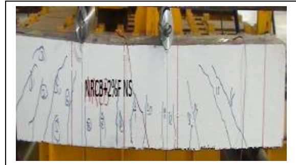
Figure 10 RC beam full shear reinforcement with 20kg/m³
