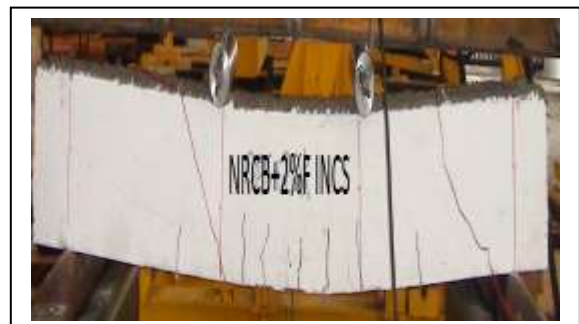
Figure 12 RC beam reduced shear reinforcement with 20kg/m³
